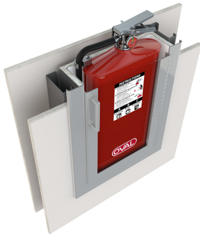
Model 10JABC shown installed in a fire-rated cabinet in a 3-5/8" studded wall
